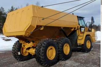
Tank: 15m<sup>3</sup> (optional 20 m<sup>3</sup>) integrated watertank with 10-20 mm reinforced epoxy coated (interior and exterior) steel walls. Hydraulic operated filling slot. Digital on-dash water level indicator. Water Cannon: Programmable, joystick controlled, durable stainless steel, also includes nozzle control. Max Capacity 15 bar, 70 meter range, 2500 L/min volume. Pump: Heavy duty hydraulic driven gunmetal housing.
